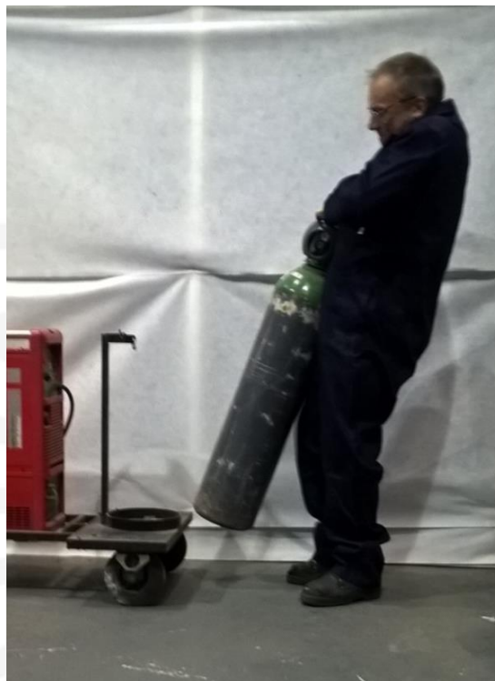
Figure 5. Manual lifting of the 63 kg cylinder onto a welding platform
