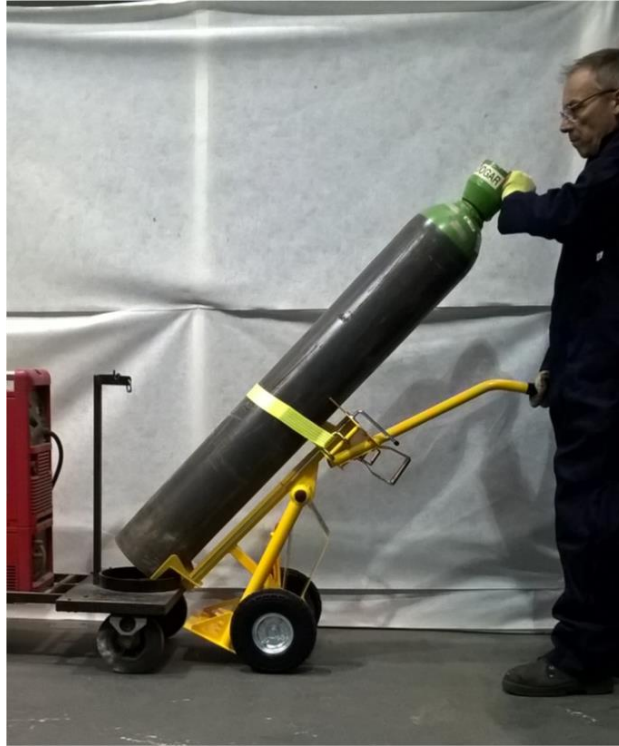
Figure 4. Loading of the 85 kg cylinder using the Cylinder Lifter onto a welding set platform
