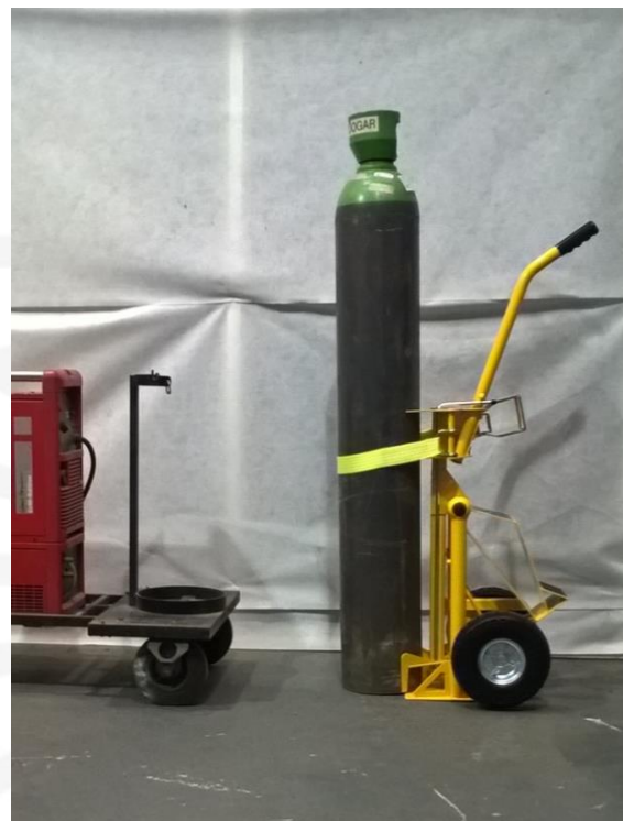
Figure 3. 85 kg cylinder ready to be lifted onto welding set platform
