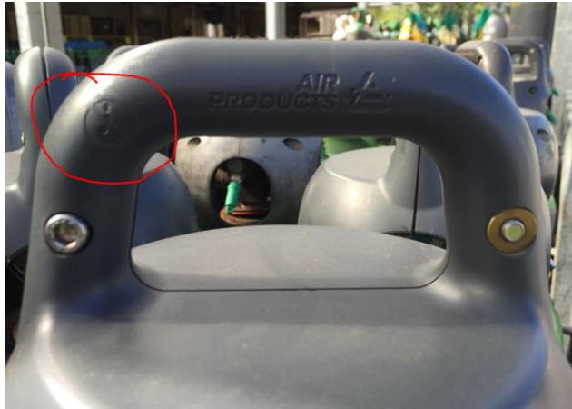
Figure 9. Handle assembly on cylinder with icon indicating that the handle is not for lifting
